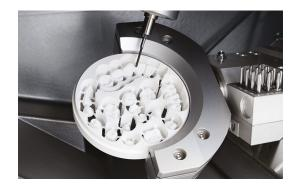
Another novelty is the integrated water cooling, which significantly minimizes the thermal expansion of the spindle and Z axis. Faster machining with even more consistent results and longer spindle lifes are the benefits for future HinriMill R5 owners.
