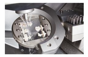
Direct Clean Technology allows you to conveniently switch between wet and dry machining. In addition to integrated ionizers and active workspace ventilation, the HinriMill R5 also has a highly intelligent drying feature.
