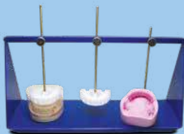
Fixation device for flaskless duplication
